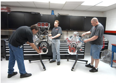
The BRE Staff Assembling Customers' Engines Prior to Dyno Tuning
