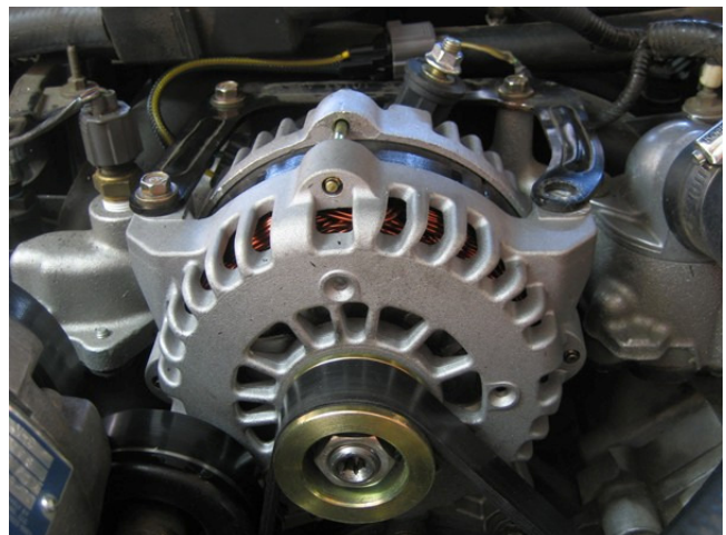
Connect the DC Power unit exactly as the OEM except the charge lead. Your unit may include an adapter harness to facilitate this.
