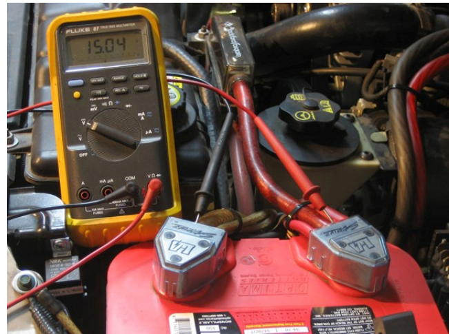
Start the engine and monitor voltage at the battery at idle. It should be in excess of 14.2 VDC. If not, see below.
