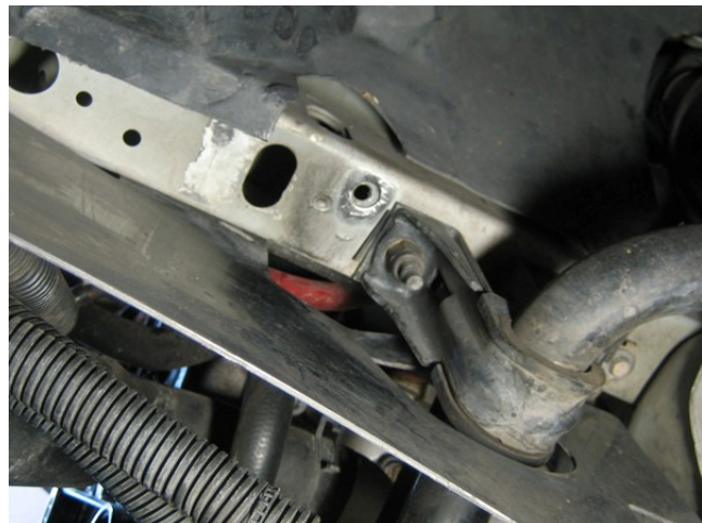
Locate an existing hole in a thick part of the subframe and tap it to accept a 5/16-18 bolt. Grind the paint to ensure a low resistance connection. Use white lithium grease to prevent rust or corrosion.
