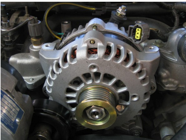
Install the DC Power high-output alternator. The unit shown is our FAD 240 – capable of 240 Amps and is internally regulated.
