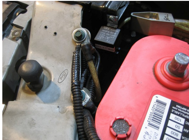
Upgrade the OEM accessory ground lead from the battery ( - ) to the chassis with an 8 AWG* lead from the battery negative ( - ).
