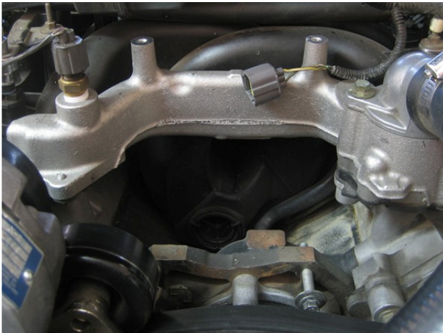
Disconnect the charge lead and plug(s) from the OEM alternator. Remove it from the vehicle.
