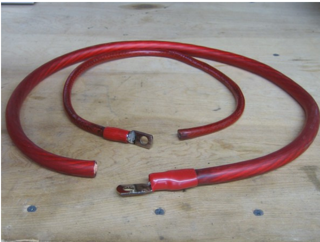
Make a new charge lead with the appropriate sized cable to go between the alternator output stud and the battery positive (+). In the case of the 240 amp unit shown, 1/0 AWG* cable is required. Solder or crimp ring terminal(s) to the end of the charge lead.
