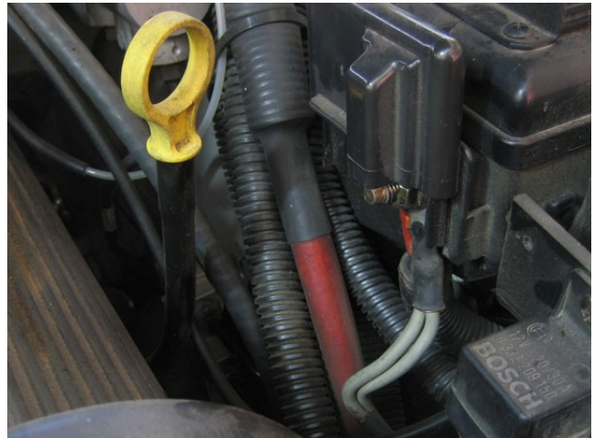
The stock charge lead runs to the under hood fuse box. A jumper from this point connects the charge lead to the battery positive ( + ).
