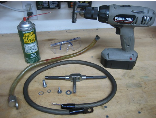
Shown are the tools required when upgrading the return path of full frame or Unibody vehicles. Make up appropriate sized cables to upgrade the return path of the alternator and battery negative ( - ).
