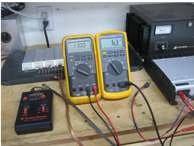
11.00 VDC = 6.3 Amps of input current
