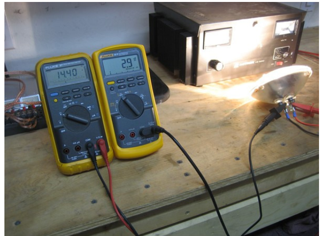
14.40 VDC = 2.9 Amps of input current
