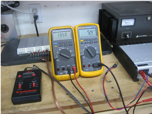
13.50 VDC = 5.4 Amps of input current
