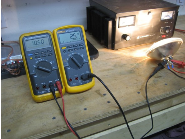
10.50 VDC = 2.5 Amps of input current
