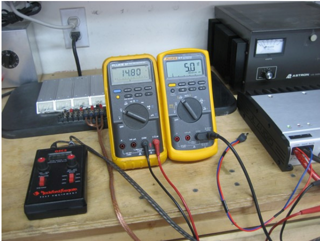
14.80 VDC = 5.0 Amps of input current
