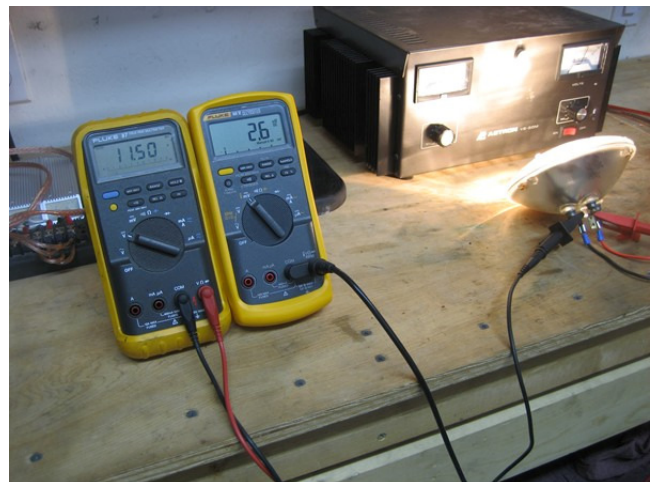
11.50 VDC = 2.6 Amps of input current
