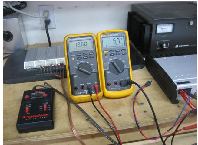
12.60 VDC = 5.7 Amps of input current
