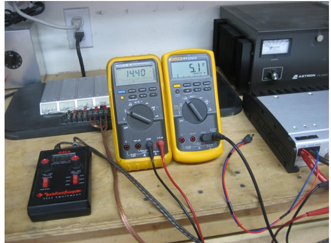
14.40 VDC = 5.1 amps of input current
